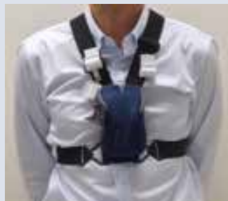
Personal wearable exposure monitors: MicroPEM™ and Ogawa™ badges.
